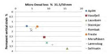
Figure 4.32 Permanent vertical strain from triaxial tests (dry) compared with micro-Deval results. Regression coefficient R<sup>2</sup> is 0.83. R<sup>2</sup> is 0.88 without Freste which can be an outlier (medium grained)
