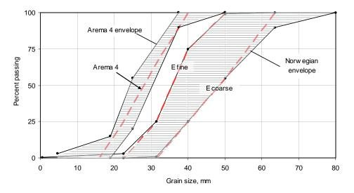
Figure 3 Grain size distribution curves for the three single-graded railway ballast samples used in this project (broken line).
