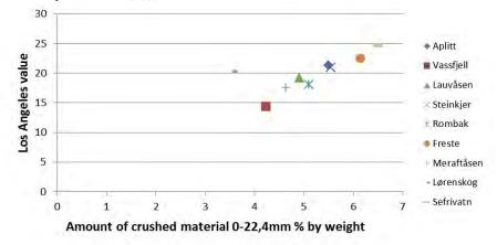
Figure 7: LAA values (10-14 mm) plotted against breakage from triaxial tests performed in wet state (4 million loadings). R<sup>2</sup> without Lørenskog is 0.97.
