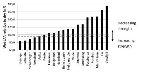
Figure 4.7 Los Angeles abrasion values (31.5/50 mm) of water saturated rocks in per cent of the strength (LAA) of air-dried rocks. Dotted lines suggest one standard deviation (average).
