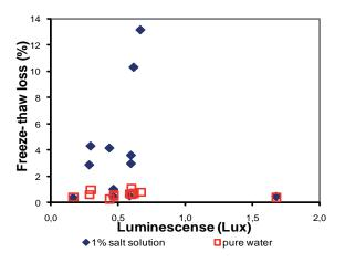
Figure 6: Graphical plot between freeze-thaw loss and luminescence.
