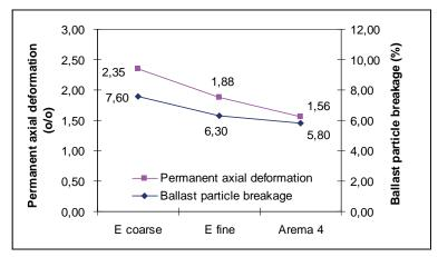
Figure 10 Permanent axial deformation compared to amount of ballast particle breakage smaller than Dmin in test specimen.
