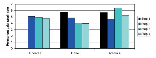
Figure 5 The correlation between permanent axial strain rate and number of test steps. Data from E coarse step 1 was not recorded.
