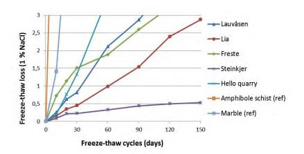
Figure 4.16 Example of long term recording of frost resistance in 1 % NaCl solution. Freeze-thaw loss in % of dry weight. Fraction 8/16 mm and 1 kg sample weight.
