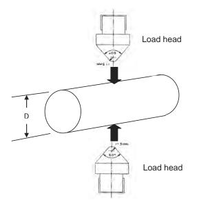
Figure 2.8 Point Load test on drilled cores from rocks. Diameter D was 50 mm.
