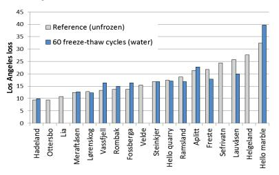
Figure 4.19 Los Angeles abrasion test run on aggregates (31.5/50 mm) after subjected to 60 freeze-thaw cycles.
