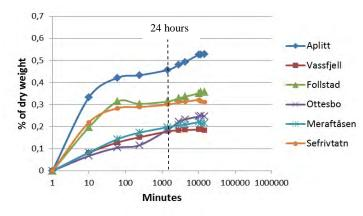
Figure 4.40 Absorption of water on drilled cores. No vacuum used. Test finished after 10 days (Bjerga 2011).
