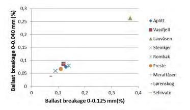
Figure 4.38 Ballast breakage from full scale railway track model test. Original grading 22.4/63 mm. Correlation between fraction 0/0.040 mm and 0/0.125 mm. R<sup>2</sup> = 0.985
