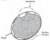
Figure 1: Key morphological properties of an aggregate particle (Pan and Tutumluer 2005).
