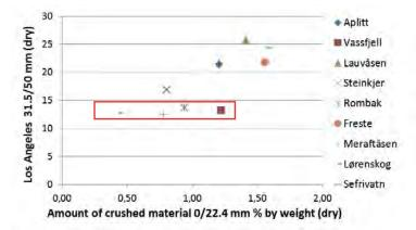
Figure 4.26 Total amount of crushed material from full scale model test (4x1 million loadings and dry state) related to mechanical strength (LAA dry). R<sup>2</sup> =0.64.
