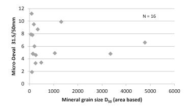
Figure 8: Mineral grain size  $D_{50}$  based on grain area plotted against micro-Deval (mechanical strength). Test results from alternative fraction Micro-Deval  $_{10/14mm}$  gave fairly the same correlation.
