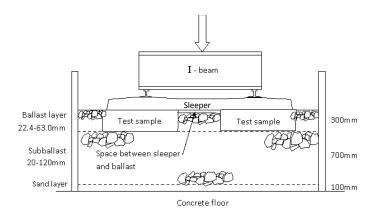
Figure 3: Cross-section of the full scale rail track model test setup.
