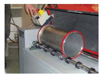
Figure 2.7 The micro-Deval test cylinder for fraction 31.5/50 mm ballast.
