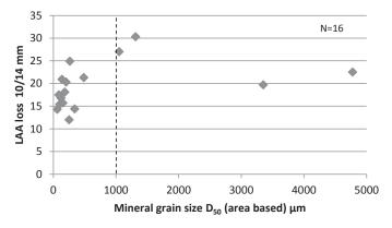
Figure 7: Mineral grain size D<sub>50</sub> based on grain area plotted against LAA<sub>10/14mm</sub> (mechanical strength) loss. Most samples were crystalline rocks and are constituted of mainly hard minerals.
