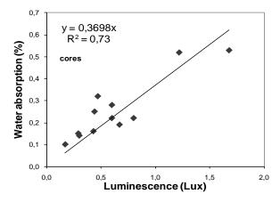
Figure 4.39 A graphic plot between luminescence and water absorption from drilled cores.
