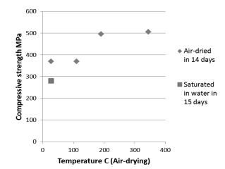
strength of 12 % (-4 to -20 %). This experience shows that oven-drying of test specimens can change the rocks' original mechanical strength.
