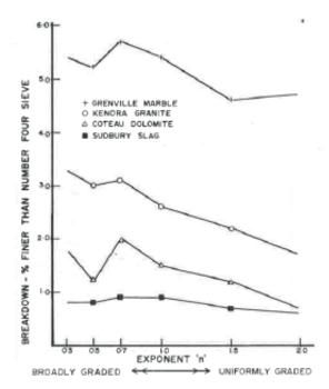
Figure 4.22 Variation in ballast breakage with gradation and with mechanical strength (Raymond 1977b). Number four sieve has 4.75 mm openings.
