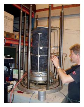
Figure 2 Instrumentation of a sample in the triaxial test rig
