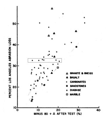
Figure 4.36 Production of fines versus Los Angeles abrasion loss for several rock types. Sieved on sieve no. 80 (0.178 mm). Modified after West et al. 1970.
