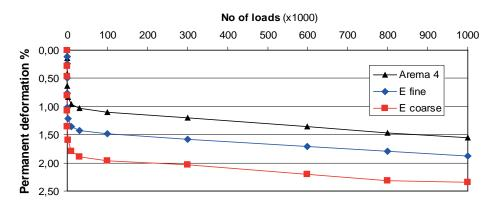
Figure 6 Permanent vertical deformation against number of loads. Each curve represents the average of four steps, totally 4 x 1 million loadings (average of three steps for grading E coarse).
