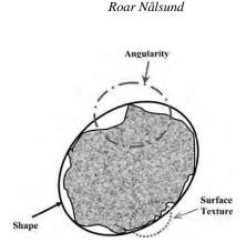
Figure 2.12 Key morphological properties of an aggregate particle. (Pan and Tutumluer 2005).
