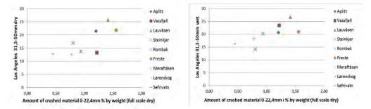
Figure 9: Total amount of crushed material from full scale model test (4x1 million loadings /only dry state) plotted against LAA<sub>31.5-50mm</sub>. Left: dry state with  $R^2 = 0.56$ . Right: wet state with  $R^2 = 0.58$ , but increase to 0.73 when Freste (medium grained) is removed.
