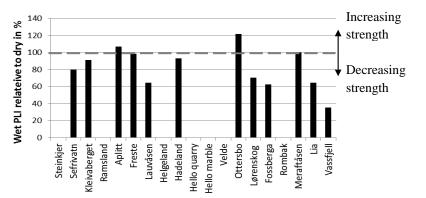
**Figure 4.9** Point Load Index (Is<sub>50</sub>) or tensile strength for water saturated rocks in per cent of the strength of air dried rocks. Drilled core diameter was 50 mm.
