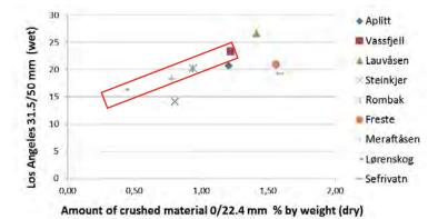
Figure 4.27 Total amount of crushed material from full scale model test (4x1 million loadings (dry state) related to mechanical strength (LAA<sub>31.5/50 m</sub>wet). R<sup>2</sup>=0.41.
