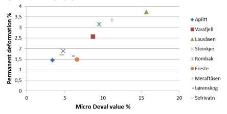
Figure 8: Ballast permanent deformation from dry triaxial tests (4x1mill loadings) plotted against micro-Deval values (31.5-50 mm). R<sup>2</sup> is 0.86 with Lauvåsen included.
