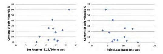
Figure 4.11 Relation between rocks' content of soft minerals and mechanical strength (wet state). Left: Los Angeles 31.5/50 mm wet. Right: Point Load Index Is<sub>50</sub> wet.
