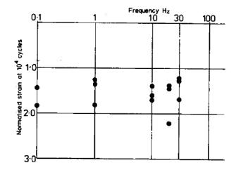
Figure 2.19 The permanent axial strain produced by 10<sup>4</sup> load cycles is plotted against loading frequency (Shenton 1975).
