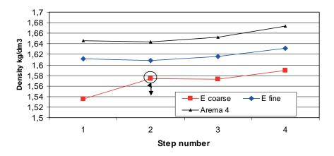
Figure 7 Change in the specimen density from step 1 to step 4. The measures are taken after each preconditioning (compaction in the steel mould) but before the loading sequence.
