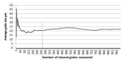
Figure 2: The plot shows the relation between calculated average mineral grain size (arithmetic) and the number of grains counted (Steinkjer quarry). Note that average grain size is stable after approximately 250 measurements.
