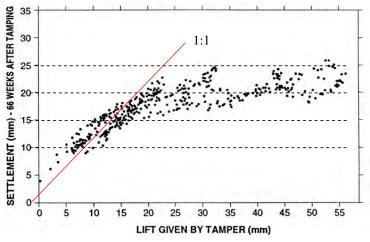
Figure 6.3 Measurement of sleeper settlements 66 weeks after tamping as a function of tamping lift (modified after Selig and Waters 1994).
