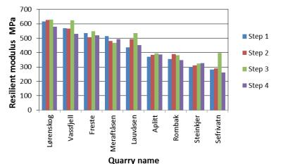
Figure 4.1 Elastic properties (dry state) to nine different rock types. Number of loadings are 1 million for each step.
