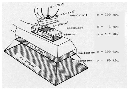
Figure 1.2. Example of pressure distribution from wheel/rail interface down to ballast/subballast interface (modified after Esveld 1989/ Führer 1978).
