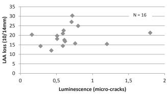
Figure 9: Luminescence against LAA<sub>10/14mm</sub> loss (mechanical strength). Test results from alternative fraction LAA<sub>31,5/50 mm</sub> gave fairly the same correlation.
