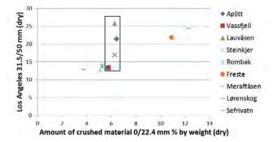
Figure 4.28 Total amount of crushed material from triaxial testing (4x1 million loadings (dry state) related to mechanical strength (LAA<sub>31.5/50 mm</sub>dry). R<sup>2</sup>=0.77.
