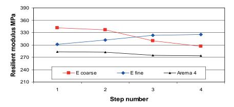
Figure 8 Change in resilient modulus from step 1 to step 4 for three different gradings. Each value is recorded at the end of each step (1 million loads). The average value for each grading is: E coarse 321 kPa, E fine 315 kPa, and Arema 4 is 278 kPa.
