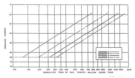
Figure 6.8 Cumulative tons of rail traffic versus ballast's mechanical strength (Clifton et al. 1987).
