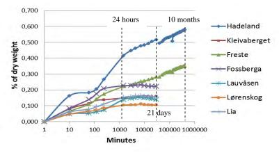
Figure 4.41 Absorption of water on drilled cores. No vacuum used.
