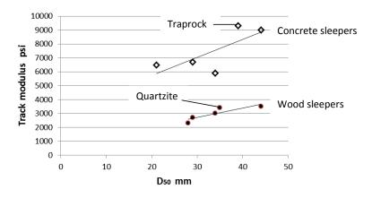
Figure 4.5 Variation in track modulus with ballast particle size. Regression coeffisient R<sup>2</sup> for concrete sleepers is 0.55 and for wood sleepers 0.77. Test materials are different types of granite with two exceptions. 1 psi = 6.89 kPa. Modified after Bosserman 1981.
