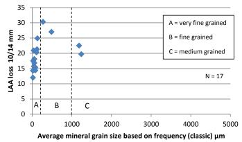
Figure 6: Average mineral grain size (arithmetic) based on grain frequency (classic calculation) plotted against LAA<sub>10-14mm</sub>. Most samples were crystalline rocks and constituted of mainly hard minerals.
