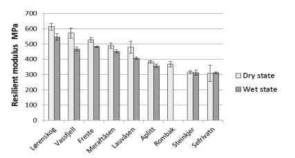
Figure 4.3 Resilient modulus of cyclic triaxial tests in dry and wet state (average of four tests). One standard deviation (+ / -) is added to the columns.
