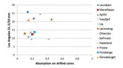
Figure 4.42 Correlation between dry Los Angeles abrasion loss <sub>31.5/50 m</sub> test and water absorption (24h) for drilled cores.
