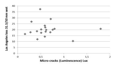
Figure 4.43 Influence of luminescense (micro-cracks) on mechanical strength (Los Angeles abrasion loss, wet state).
