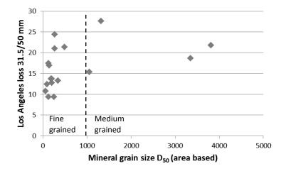
strength and mineral grain size. We did not get any improved relationship when  $D_{50}$  was replaced by frequency based average mineral grain size (Paper IV).
