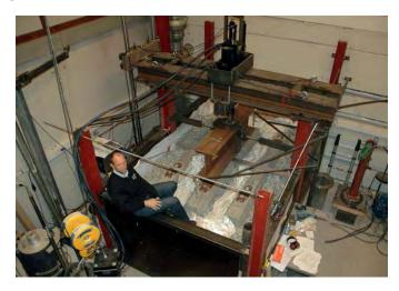
Figure 2: Full scale rail track model test setup for cyclic loading.
