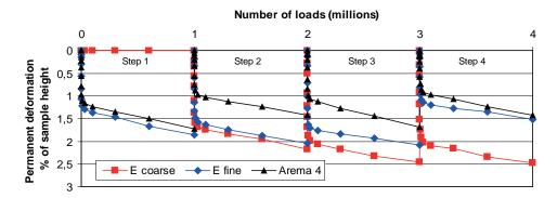
Figure 4 Permanent deformation against number of loads. Each of the three different gradings (E coarse, etc) was divided into four steps and totally subjected to 4 million load applications. Data from step 1 for grading E coarse was unintentionally not recorded.
