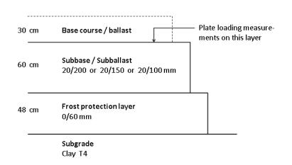
Figure 6.5 Vertical cross section of the design of Highway E6 between Trondheim and Stjørdal.
