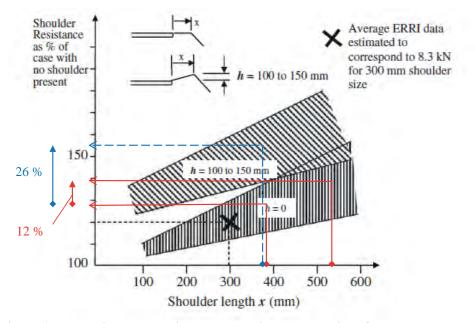
Figure 6.7 Track's lateral resistance depending on the design of the ballast shoulder (modified after ERRI 1995).
