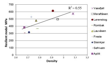
Figure 4.2 Relationship between ballast elastic property and rock density
