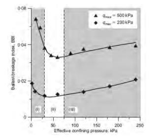
Figure 2.14 Effect of confining pressure on particle degradation at different deviatoric stress levels (Indraratna et al. 2005).
