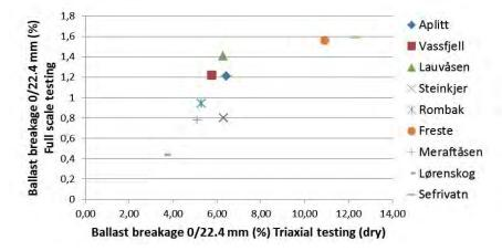
because applied vertical stiffness and confining pressure are close to the field conditions. The correlation between the two tests (both dry state) is shown in Figure 4.34.
