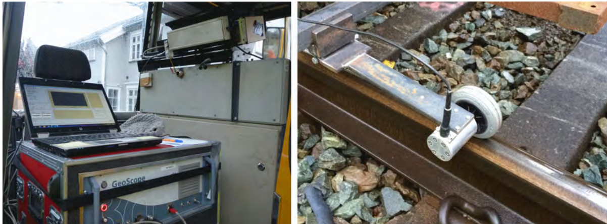
Figure 23: Left: The GeoScope radar unit and operator PC are located in the driver's cabin of the surveying vehicle. Right: Mounted rubber wheel (DMI)
