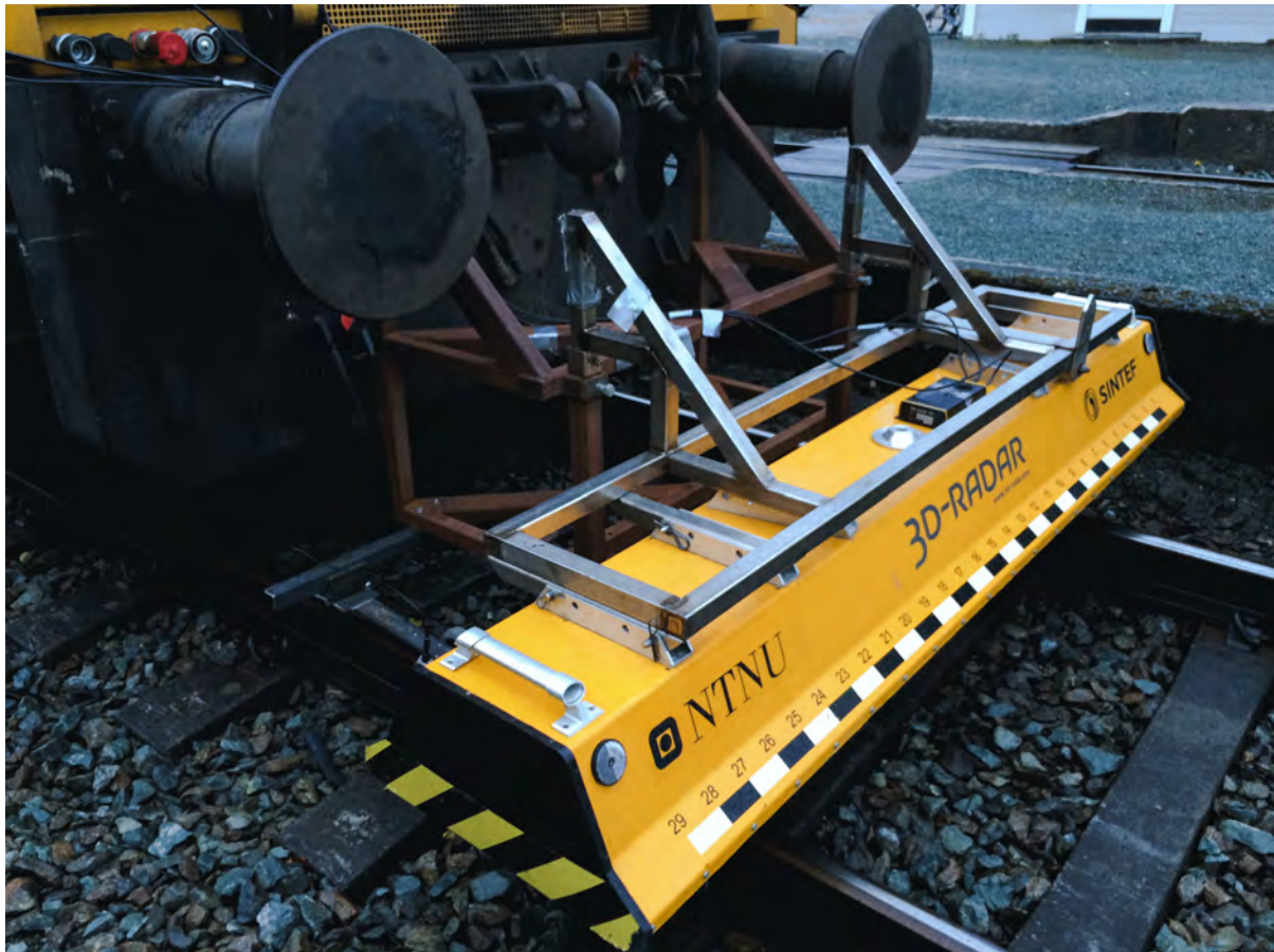
Figure 20: 3d-radar V2429 antenna-array mounted on Robel rail-tractor
