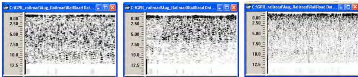
Figure 11: Scattering in radargrams with with different ballast fouling conditions. Left: Clean | Center: Partially fouled | Right: Fouled (Al-Qadi et al., 2008)
