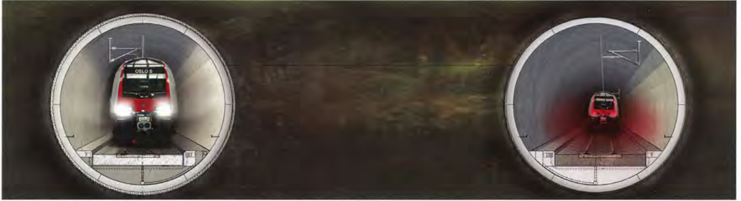
Two single bore tunnels will give the new double track line Oslo-Ski both a significant degree of flexibility and modern level of rail safety.
