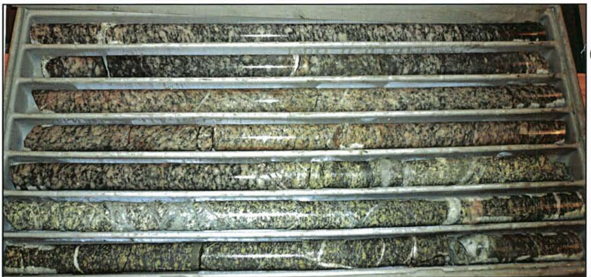
Drilled rock cores of good rock quality in upper part of the picture, and weathered rock with quartz cemented fractures below.
