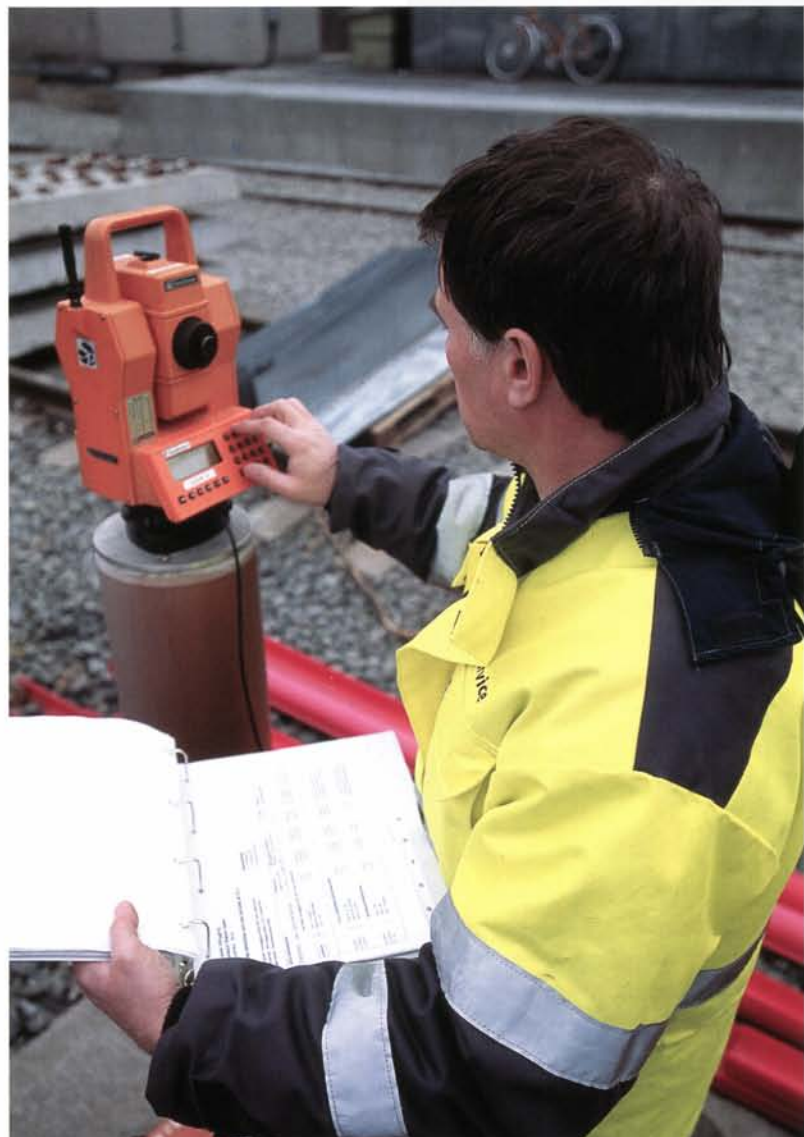
Track coordinate fixing. (Photo: Rune Fossum)
