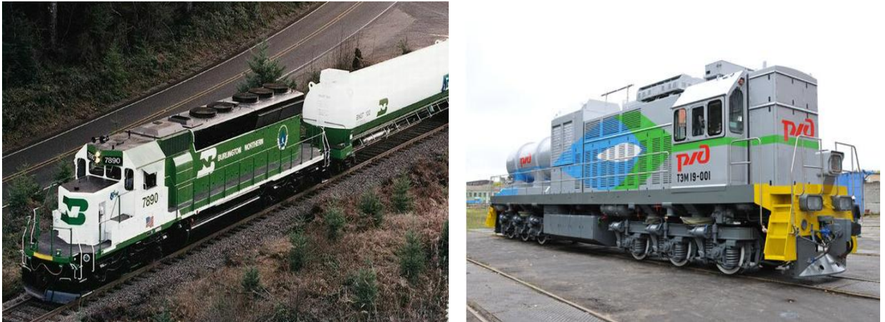
Figure 8: LNG-powered locomotive and its fuelling option (fuel tender – left side; cryogenic unit placed on locomotive – right side) (Source: Schneider 2014; Lenz 2014)
