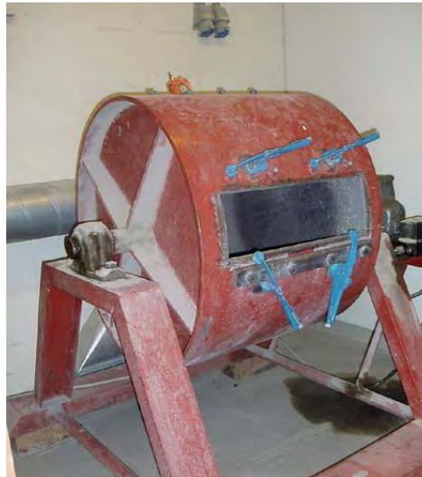
**Figure 2.5 The Los Angeles abrasion test drum without cover used for both fraction 10/14 and 31.5/50 mm. Interior diameter is 71 cm.**
