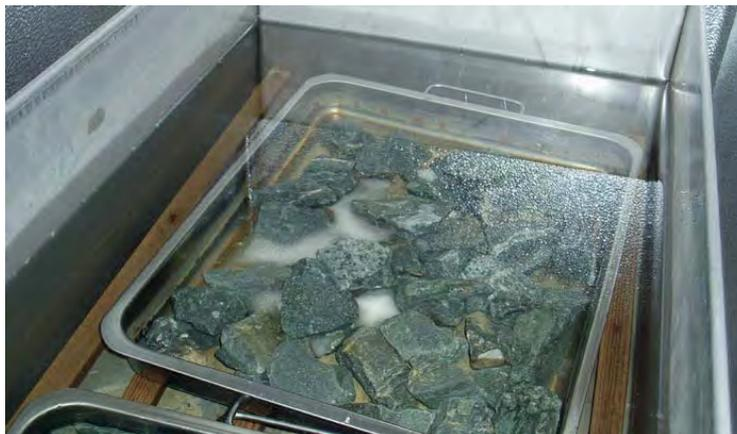
**Figure 4.20 Thawing phase of the test. Test material was soaked in water during both freezing and thawing.**
