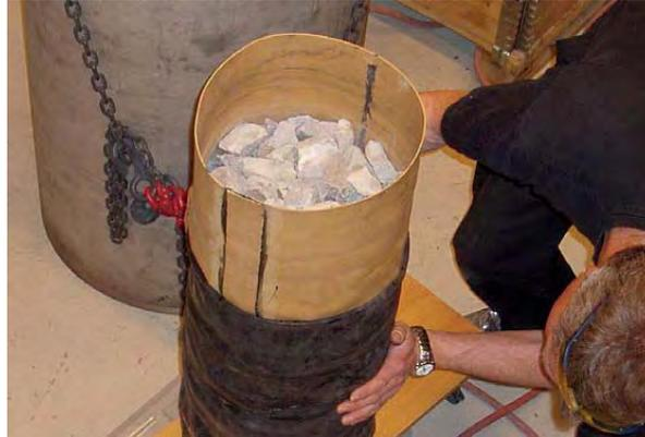
**Figure 2.17** Preparation of a test specimen.
