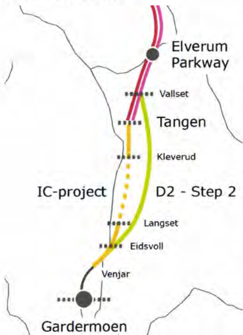
Figure 13. Østerdalen route: Construction of new double-track from Venjar and northwards starting with the IC-project (orange line) as step 1.
