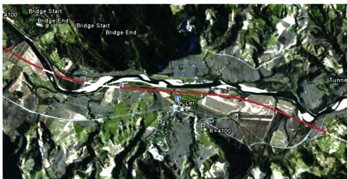
Figure 158. Two bridges crossing river Gaula close to Ler. The flooding situation will possibly require bridge viaducts adjacent to the bridges.
