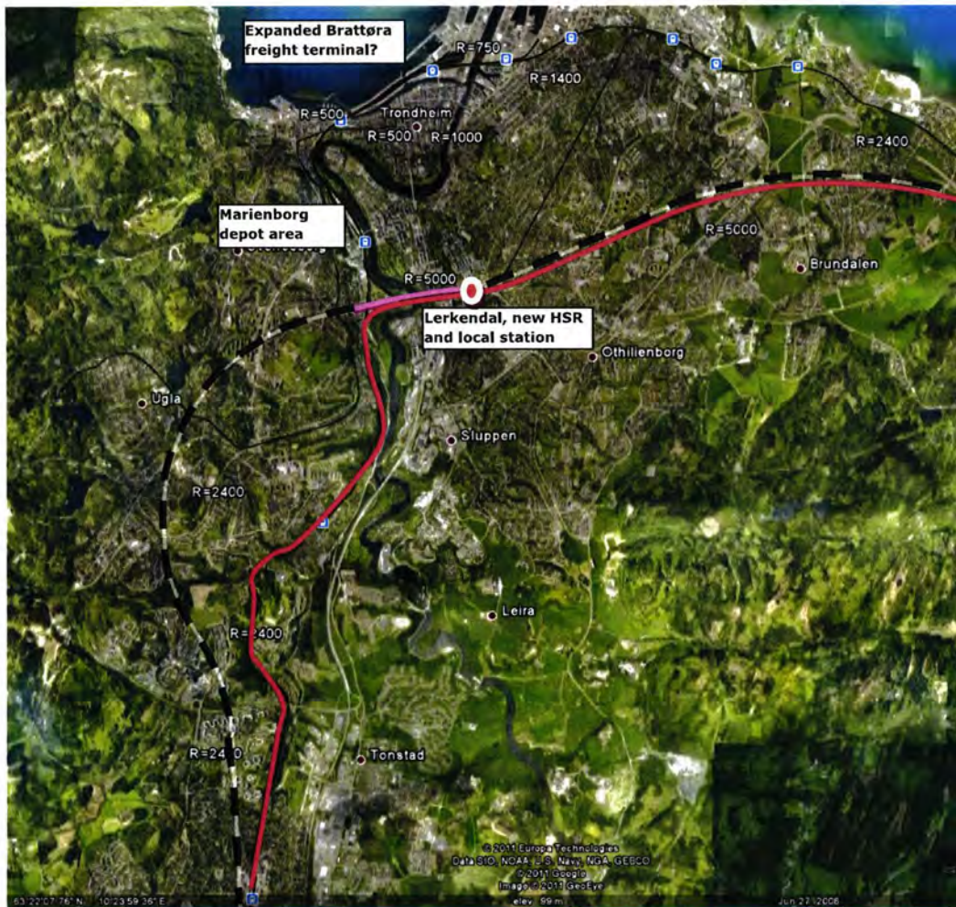
Figure 62. Possible rail-systems in Trondheim: Local rail 1 Lerkendal-Steinkjer and 2 Støren/Melhus-Stjørdal (red) and HSR Gardermoen-Trondheim-Værnes (dotted/magenta) in the same route. Source: Geovekst.
