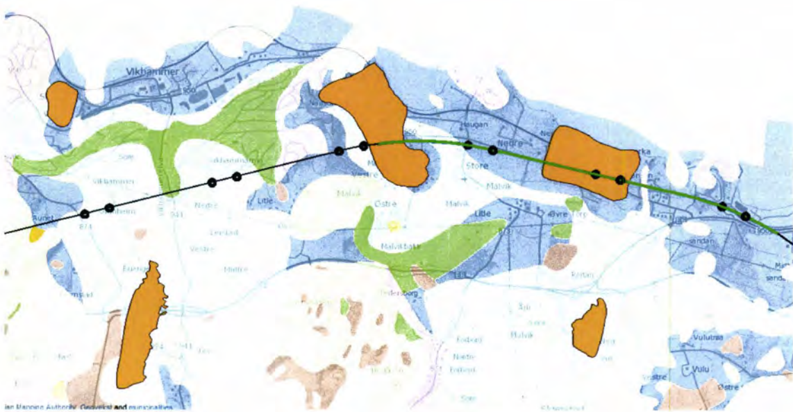
Figure 107. Difficult part (tunnel, cutting and filling) in Jonsborg quick clay zone in Malvik. Source: Geovekst. Legend see Figure 106.
