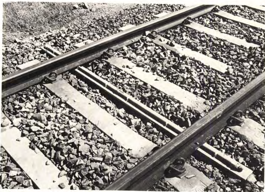
Figur 2. Indikatorstaven plassert i sporet.
