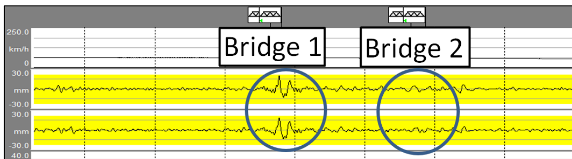
Figure 1.3 – Example: Vertical track deviations measured with ROGER 1000 at two bridges (Via Terje Vasset, Bane NOR)
