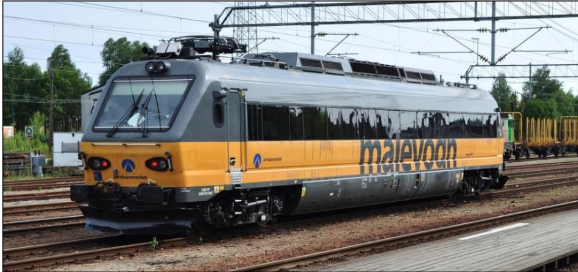
Figure 1.1 - The measuring car ROGER 1000 for controlling the entire railway network in Norway (Source www.BaneNOR.no )
