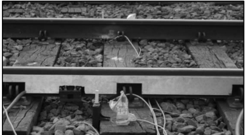
Figure 3.3 – Illustration: Placing of the geophones on top of the sleepers (From Coelho. B, 2011)
