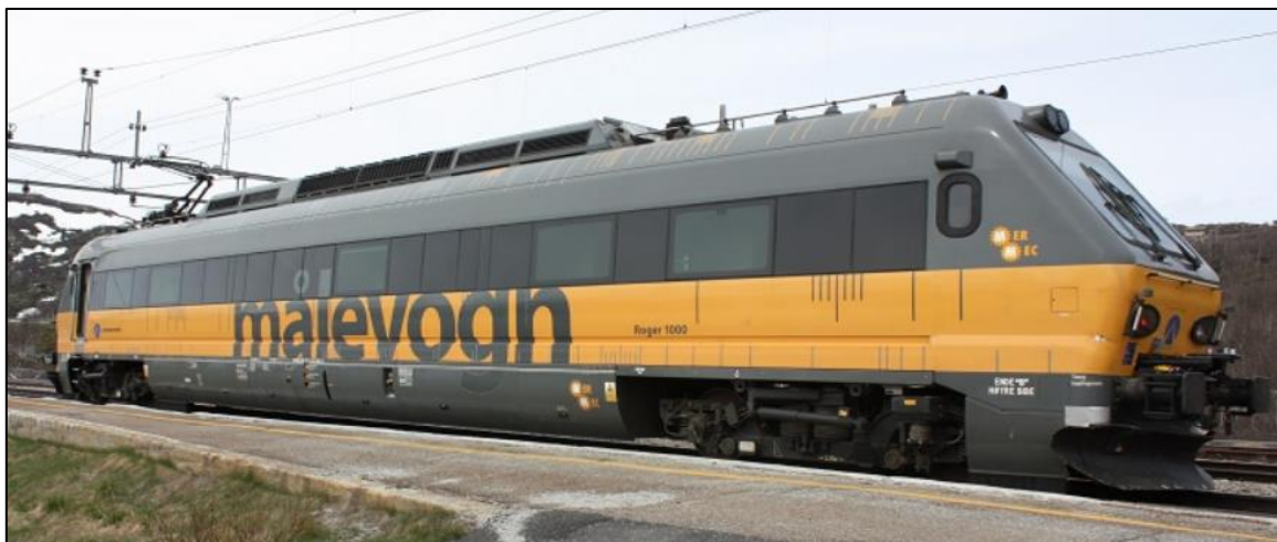
Figure 5.1 – The measuring car «ROGER 1000» used at the entire railway network in Norway (Source: www.BaneNOR.no )
