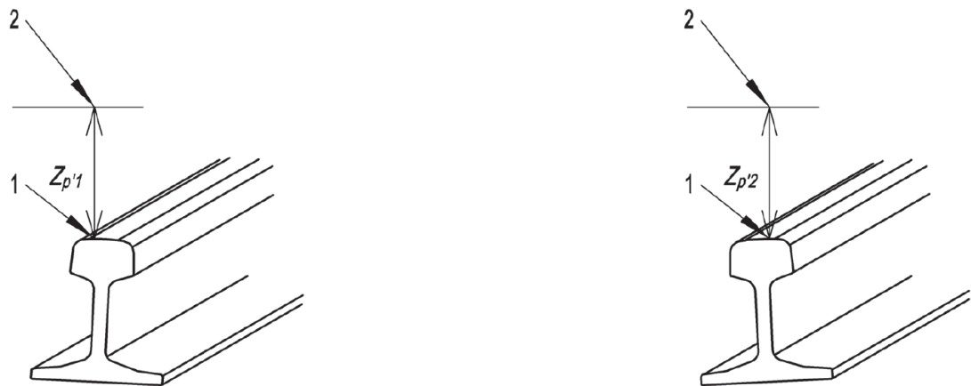
Figure 2-3 Longitudinal level (European Standard, 2008)
