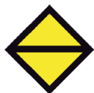
Figur 25: Signal 67 B "Orienteringssignal for planovergang"
