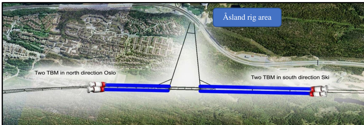
Figure 2.8 – Two TBMs are operating in each direction from Åsland rig area (Bane NOR, 2018b).
