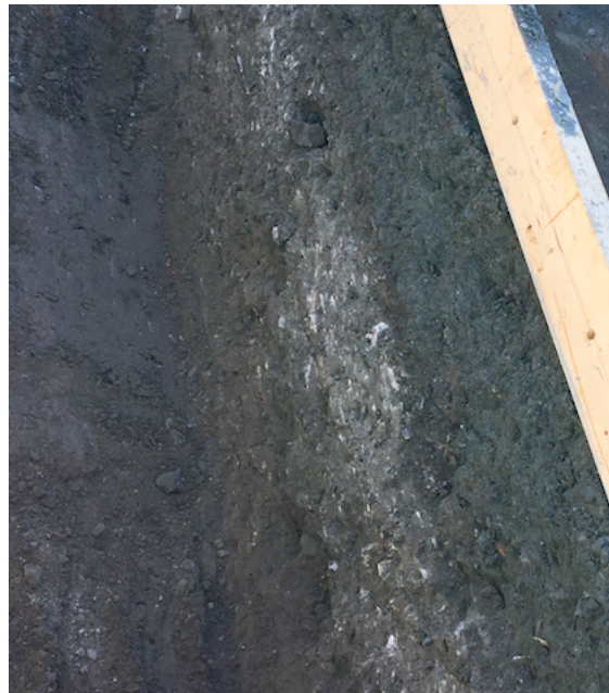
Figure 3.19 – Frozen layer discovered during field test 1, early April
