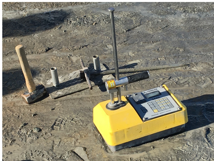
Figure 3.8 – Troxler device: The plate, hammer and nail in the background is used to make two holes for the nuclear transmitter to be lowered down to desired depth
