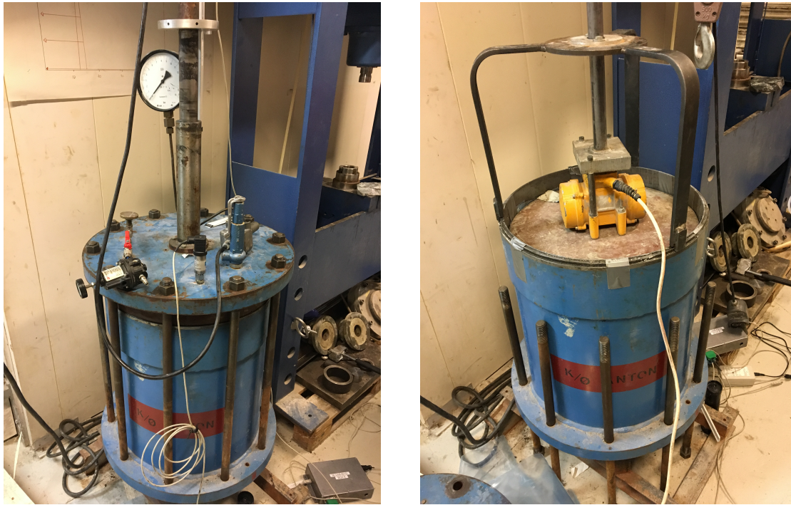
Figure 4.1 – K/Ø Anton - Equipment used for oedometer testing of TBM material. Picture to the right shows the vibrating compaction plate
