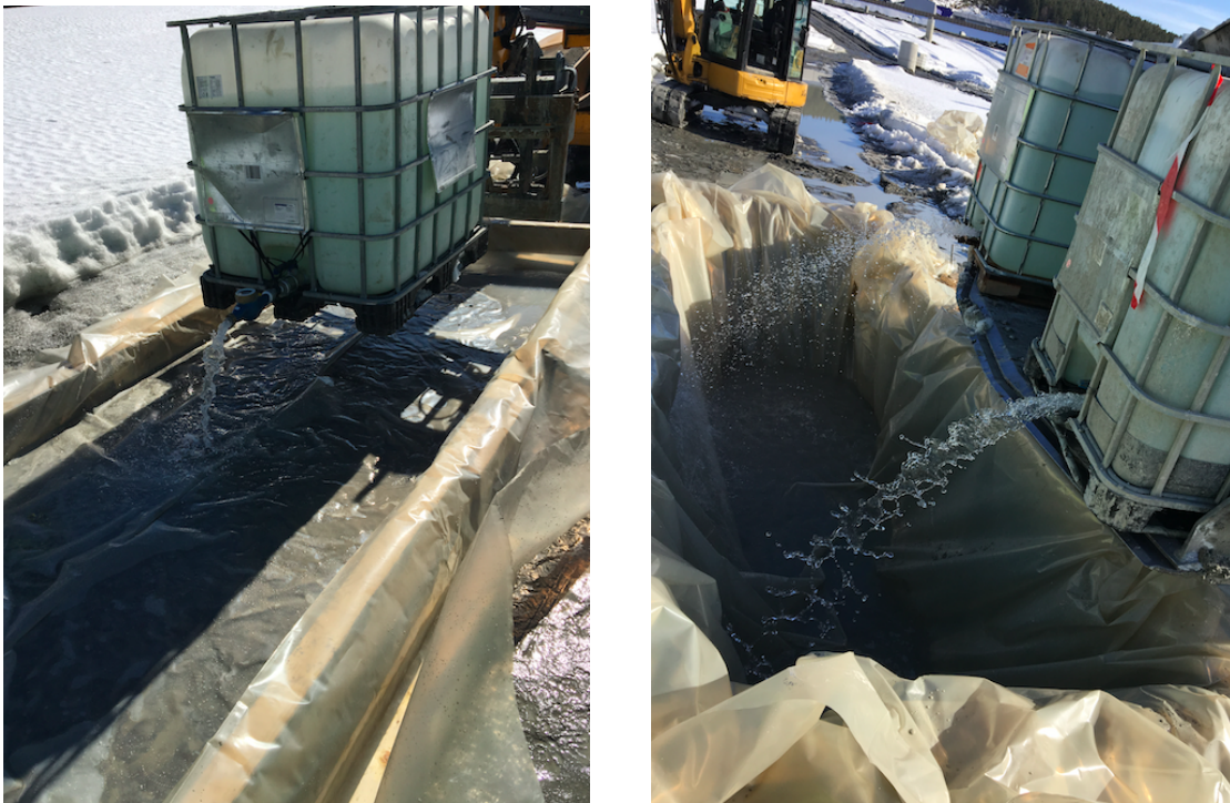
Figure 3.18 – Right: Filling frame with water, volume measured through flowmeter. Left: Pit filled with water measured as sum of several flowmeters
