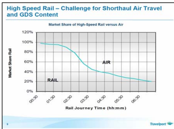
Figur 8.5: Air/rail modal split (source: Eurocontrol UIC) Analysis and modeling of passenger choice between air and rail transportation modes
