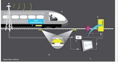
A new technology will reduce the number of signalling faults in the future. The introduction of axle counters will reduce signalling faults considerably in the short term.
